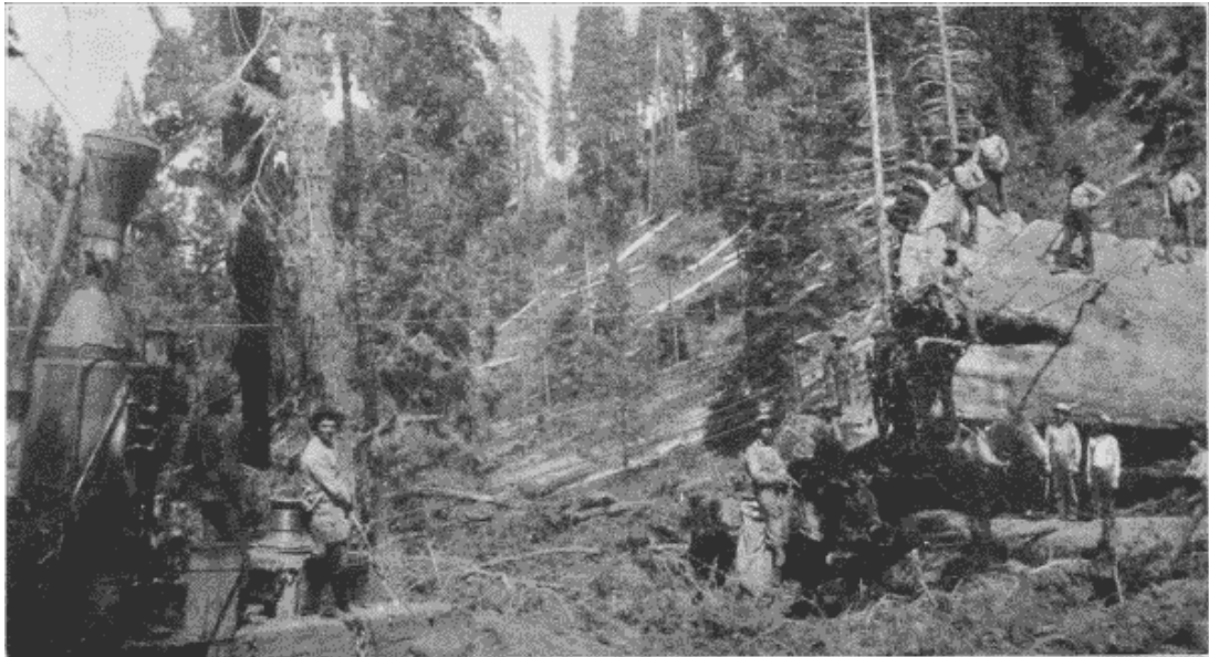
Fig. 26. Hauling Big Logs by Donkey Engine.
