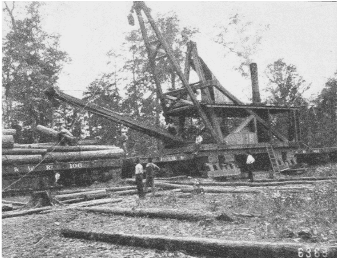
Fig. 27. Steam Skidder at Work. Grant County, Arkansas.
