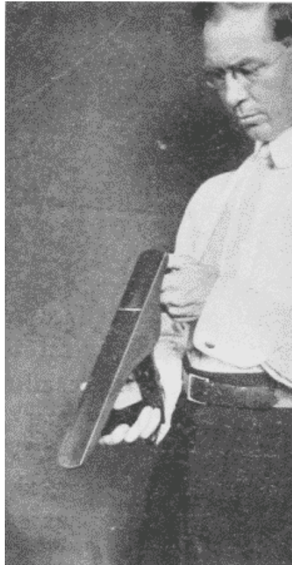
Fig. 102. Sighting Along the Sole of Jack-Plane.
