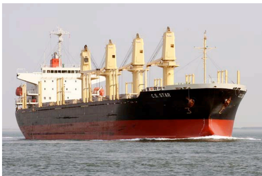
Figure 3. Dry bulk carrier, bulk freighter, or bulker, is a merchant ship used to transport unpackaged bulk cargo, such as cereals, coal, ore, and cement.
