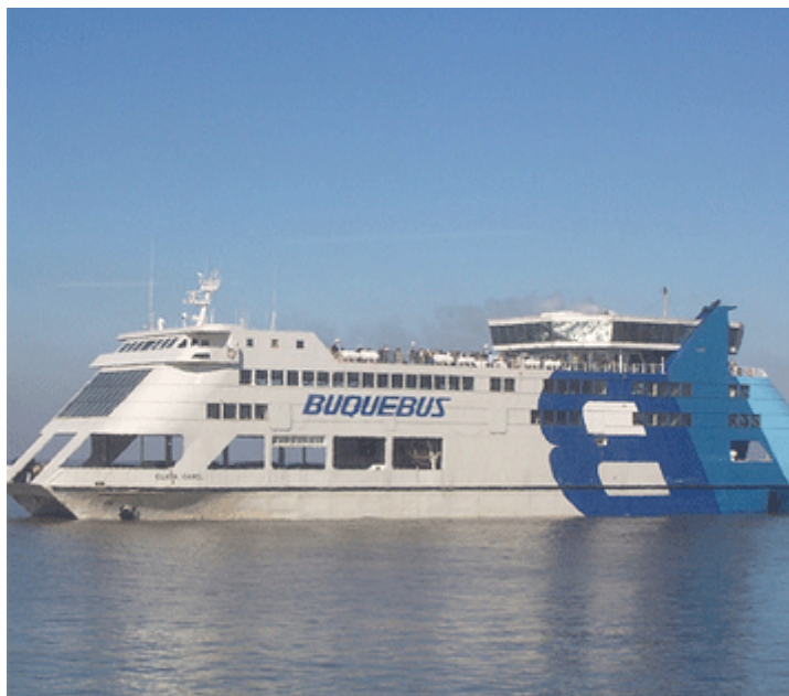
Figure 8. Passenger ferry, catamaran type
