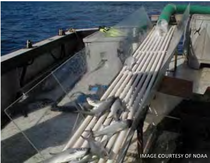
Photo of the dewatering table as fish are taken from the offshore cage in Hawaii.
