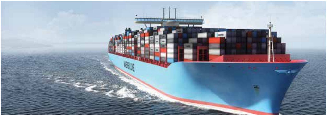
The Triple E's bridge has been brought forward so containers can be stacked higher with no loss of visibility
