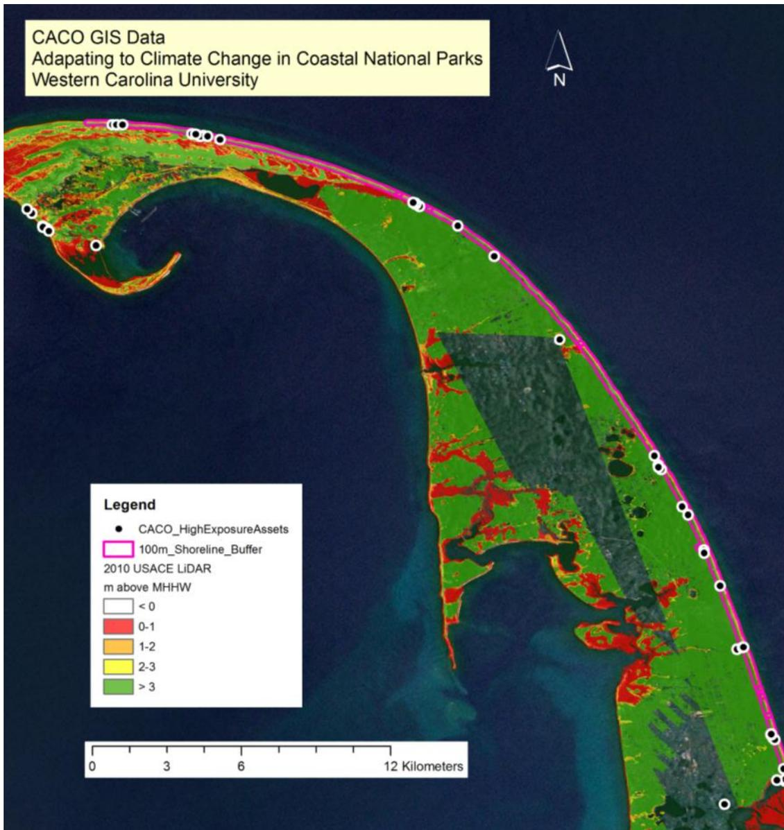
**Figure C7.** CACO GIS Map of park boundary and high-exposure assets. NOAA tides and currents website was used to calculate MHHW (0.92 m above NAVD88), for CACO used Chatham, MA station: <http://tidesandcurrents.noaa.gov/datums.html?id=8447435>.
