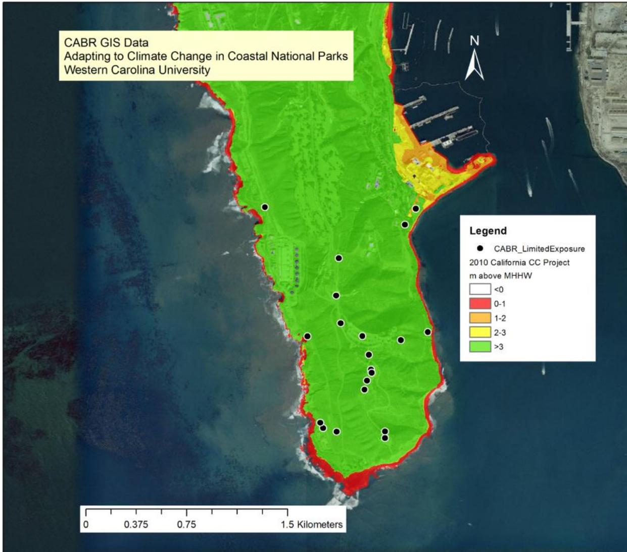
**Figure E2.** CABR GIS map of park boundary and limited exposure assets. NOAA tides and currents website was used to calculate MHHW (1.6 m above NAVD88), for CABR used La Jolla, CA station: <http://tidesandcurrents.noaa.gov/datums.html?id=9410230>.
