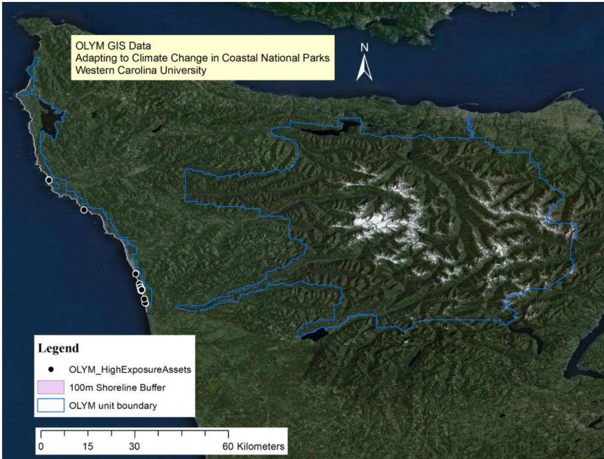
**Figure E6.**OLYM GIS map of park boundary and high-exposure assets. NOAA tides and currents website was used to calculate MHHW (2.17 m above NAVD88), for OLYM used Neah Bay, WA station: <http://tidesandcurrents.noaa.gov/datums.html?id=9443090>.
