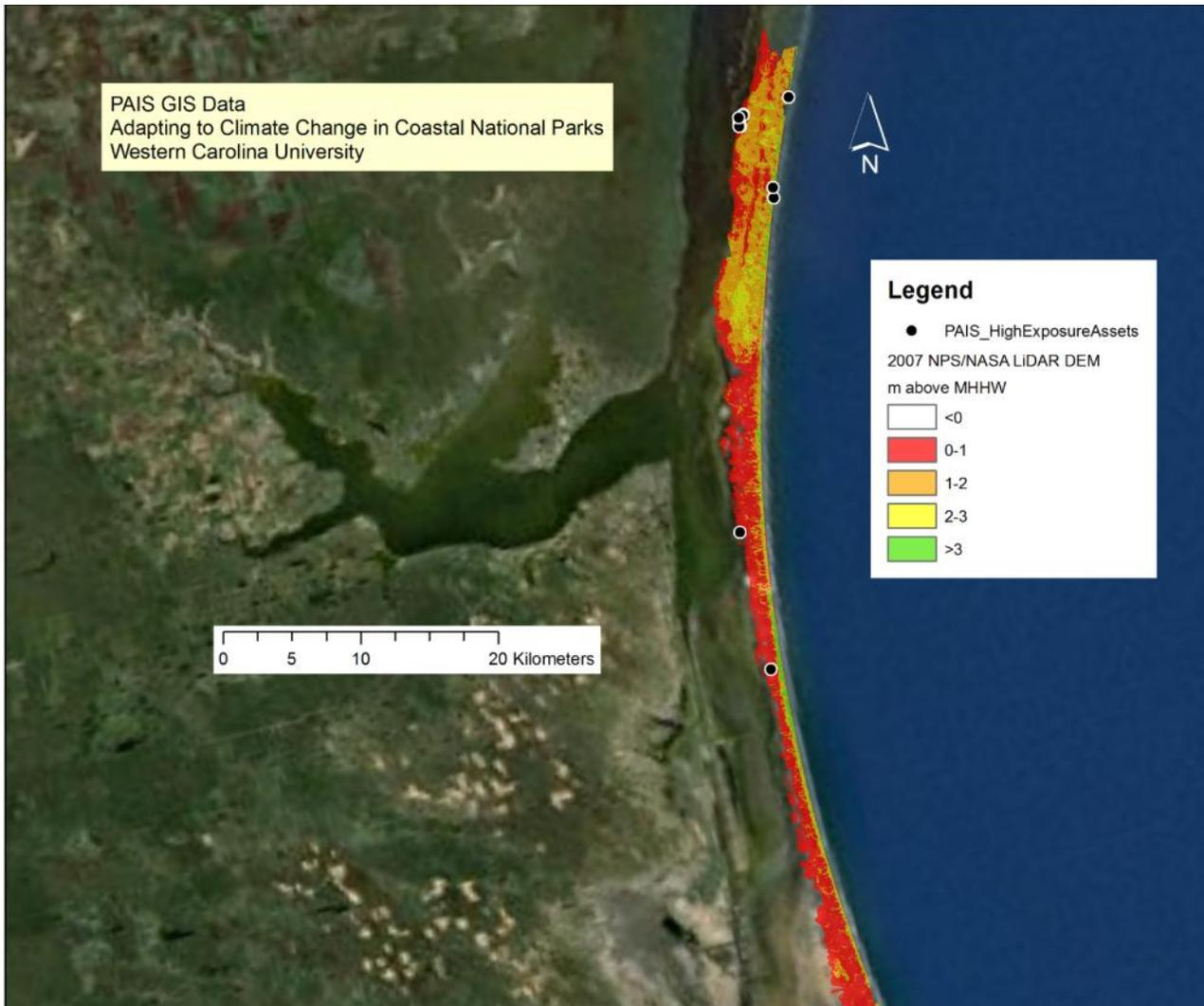
**Figure F2.** PAIS GIS map of park boundary and high-exposure assets. NOAA tides and currents website was used to calculate MHHW (0.36 m above NAVD88), for PAIS used Bob Hall Pier, Corpus Christi, TX station: <http://tidesandcurrents.noaa.gov/datums.html?id=8775870>.
