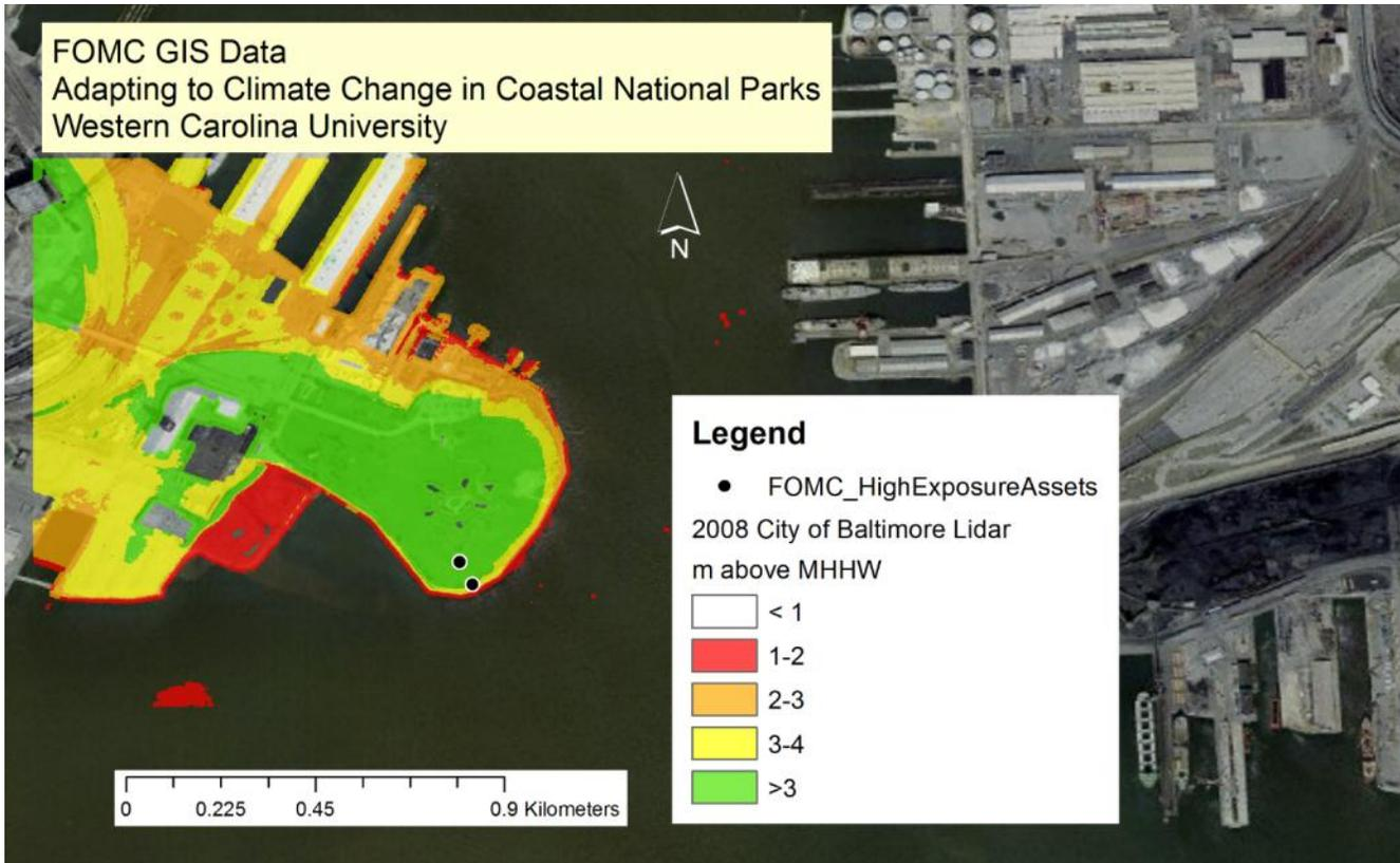
**Figure C9.** FOMC GIS Map of park boundary and high-exposure assets. NOAA tides and currents website was used to calculate MHHW (0.82 m above NAVD88), for FOMC used Baltimore, MD station: <http://tidesandcurrents.noaa.gov/datums.html?id=8574680>.
