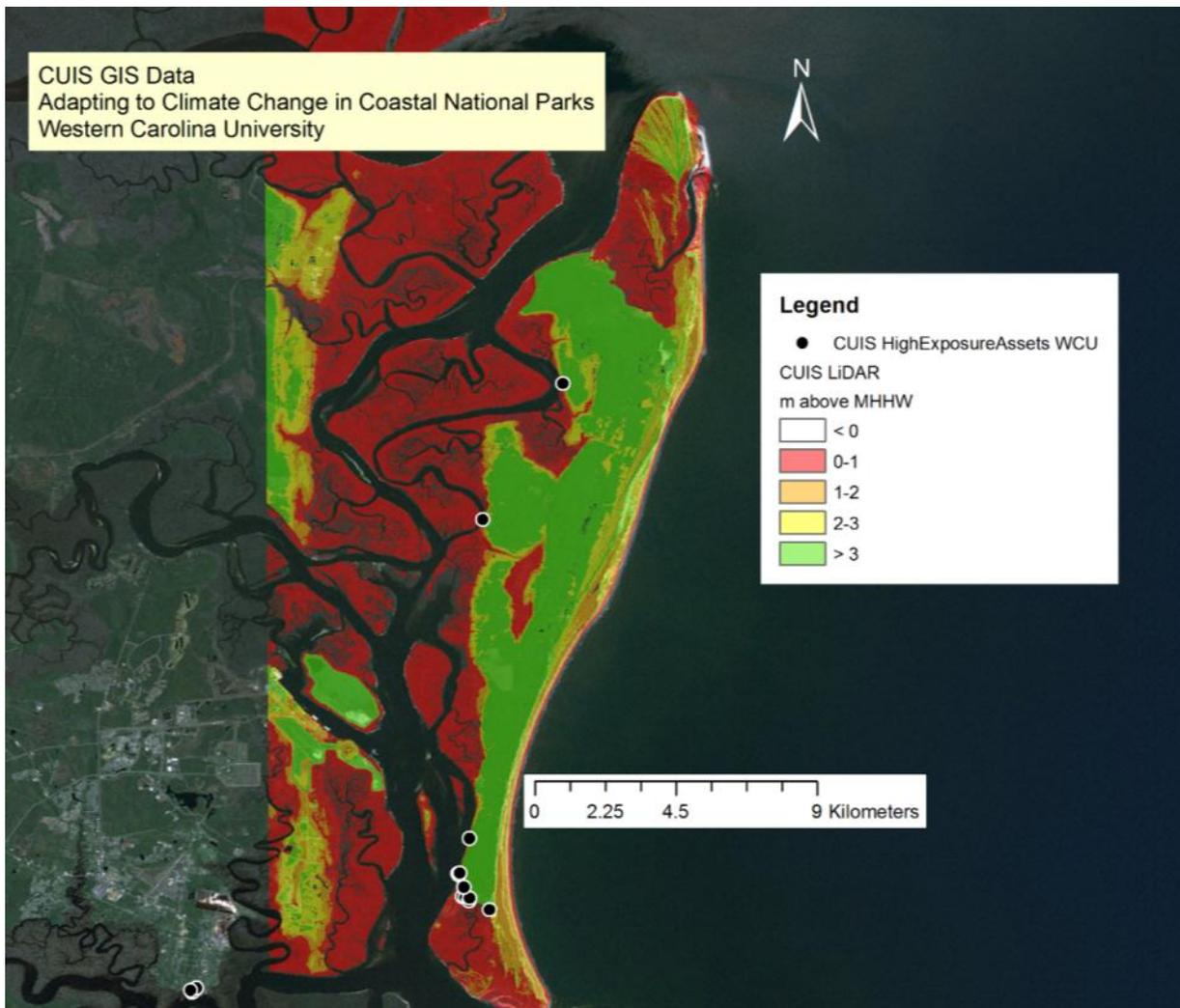
**Figure D8.** CUIS GIS map of park boundary and high-exposure assets. NOAA tides and currents website was used to calculate MHHW (0.84 m above NAVD88), for CUIS used Fernandina Beach, FL station: <http://tidesandcurrents.noaa.gov/datums.html?id=8720030>.
