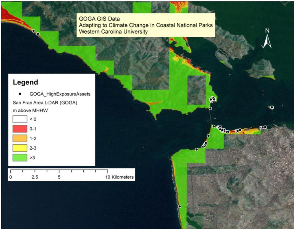
**Figure E5.** GOGA GIS map of park boundary and high-exposure assets. NOAA tides and currents website was used to calculate MHHW (1.8 m above NAVD88), for GOGA used San Francisco, CA station: <http://tidesandcurrents.noaa.gov/datums.html?id=9414290>.
