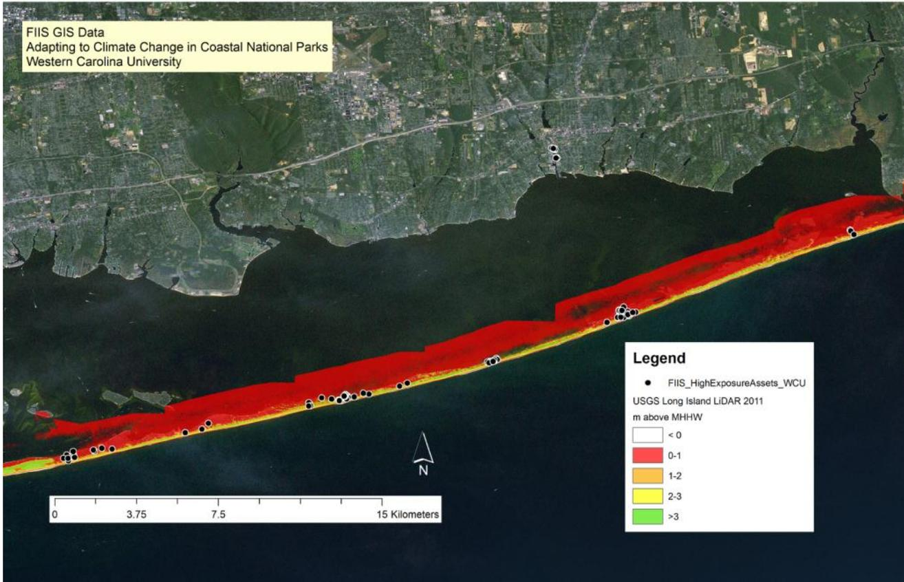
**Figure C8.** FIIS GIS Map of park boundary and high-exposure assets. NOAA tides and currents website was used to calculate MHHW (0.73 m above NAVD88), for FIIS used Sandy Hook, NJ station: <http://tidesandcurrents.noaa.gov/datums.html?id=8531680>
