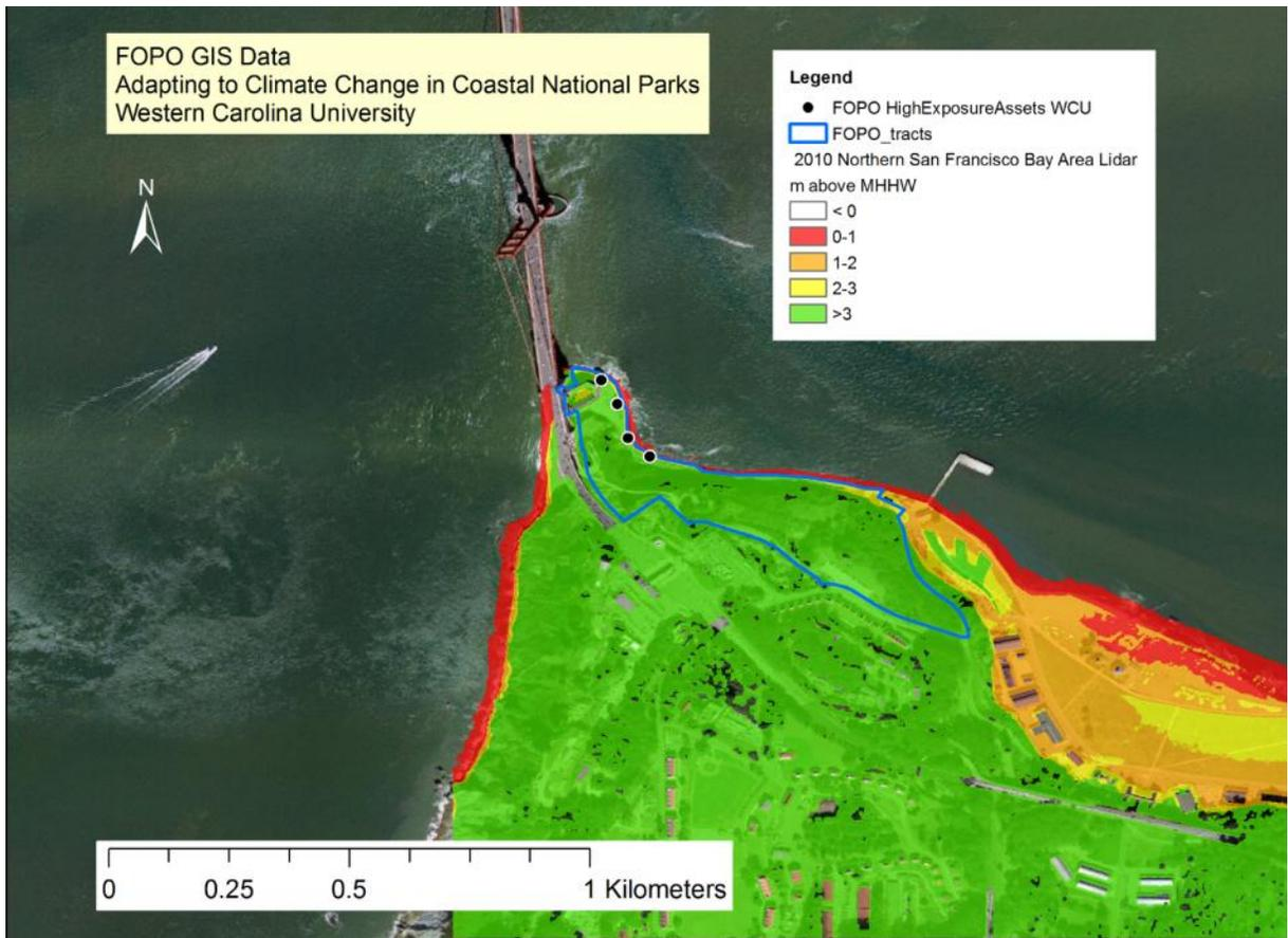
**Figure E4.** FOPO GIS map of park boundary and high-exposure assets. NOAA tides and currents website was used to calculate MHHW (1.8 m above NAVD88), for FOPO used San Francisco, CA station: <http://tidesandcurrents.noaa.gov/datums.html?id=9414290>.
