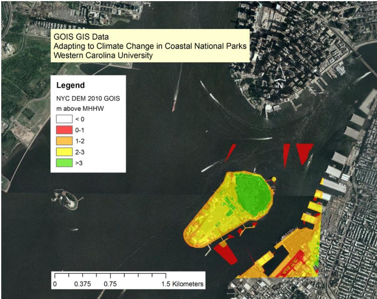
**Figure C12.** GOIS GIS Map of park boundary and high-exposure assets. NOAA tides and currents website was used to calculate MHHW, for GOIS used Battery Park, NY station: <http://tidesandcurrents.noaa.gov/datums.html?id=8518750>.
