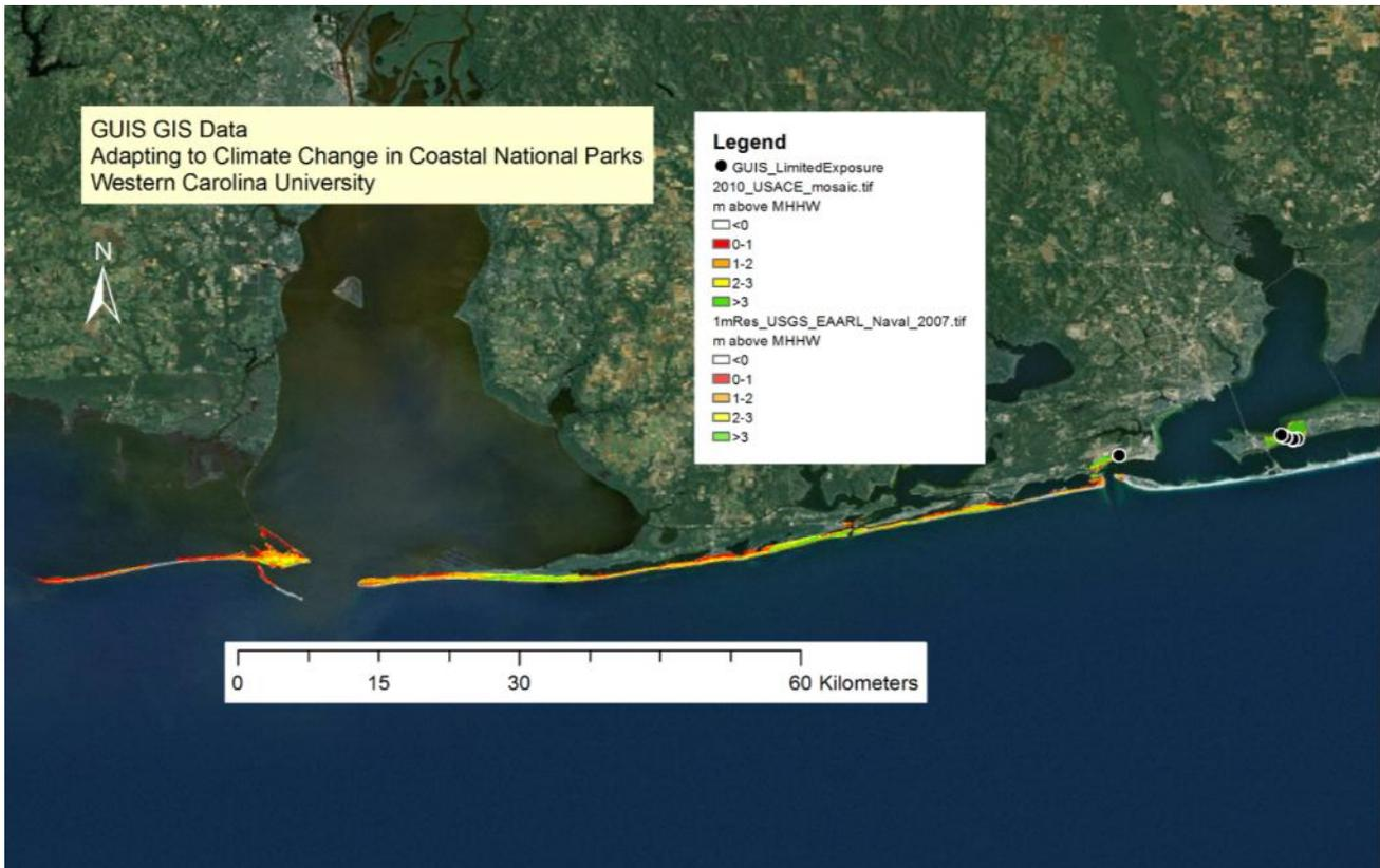
**Figure D9.** GUIIS GIS map of park boundary and limited exposure assets. NOAA tides and currents website was used to calculate MHHW (0.21 m above NAVD88), for GUIIS used Dauphin Island, FL station: <http://tidesandcurrents.noaa.gov/datums.html?id=8735180>.
