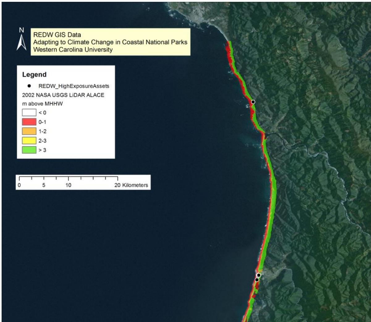
**Figure E8.** REDW GIS map of park boundary and high-exposure assets. NOAA tides and currents website was used to calculate MHHW (1.88 m above NAVD88), for REDW used Fields Landing, Humbolt Bay, CA station: <http://tidesandcurrents.noaa.gov/datums.html?id=9418723>.
