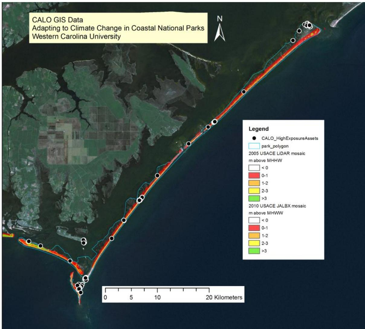
**Figure D5.** CALO GIS map of park boundary and high-exposure assets. NOAA tides and currents website was used to calculate MHHW (0.23 m above NAVD880), for CALO used Wrightsville Beach, NC <http://tidesandcurrents.noaa.gov/datums.html?id=8658163>.
