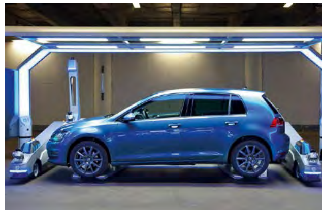
Figure 19: Ray – an automated system that improves parking space utilization by 60 %; Source: MV Media
