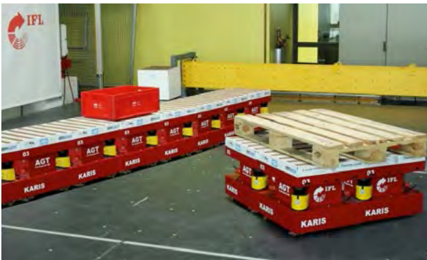
Figure 32: Small autonomous vehicles in the KARIS PRO System; Source: Karlsruher Institut für Technologie
