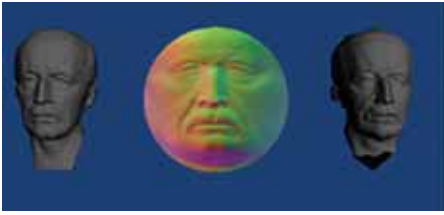
Real time projection of a head model onto a sphere and the resulting reconstruction.
