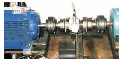
Laboratory prototype BDFG (left) on test rig with torque transducer and DC load machine (right)
